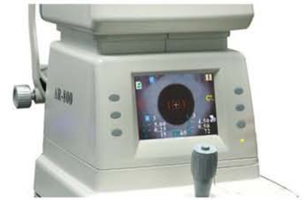
An autorefractor is performed to verify or update your prescription measurements for contact lenses.
